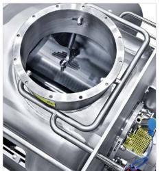
Cleaning nozzles for the WIP process
