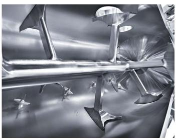
Welded mixing elements in hygienic design
