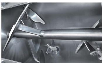
Mixing tools welded onto the main shaft in hygienic design
