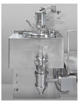
MGT with downstream sieve mill
