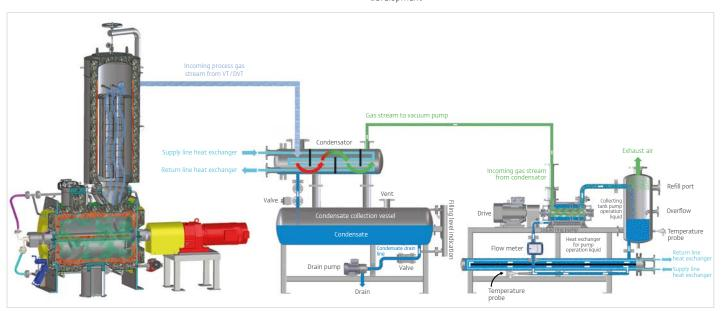
Principle of the DRUVATHERM® Vacuum Shovel Dryer
