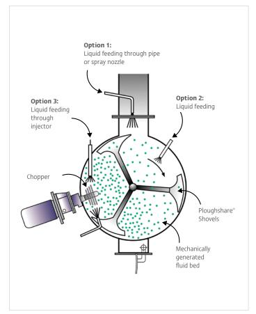
Some liquid addition possibilities in the LÖDIGE Ploughshare® Mixer following the principle of the mechanically generated fluid bed
