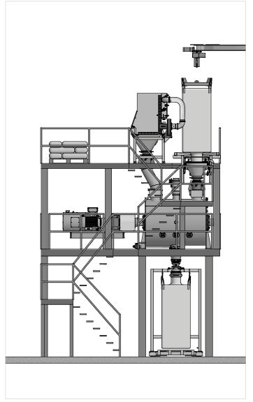
Mixing plant with manual infeed, big bag feeding and filling
